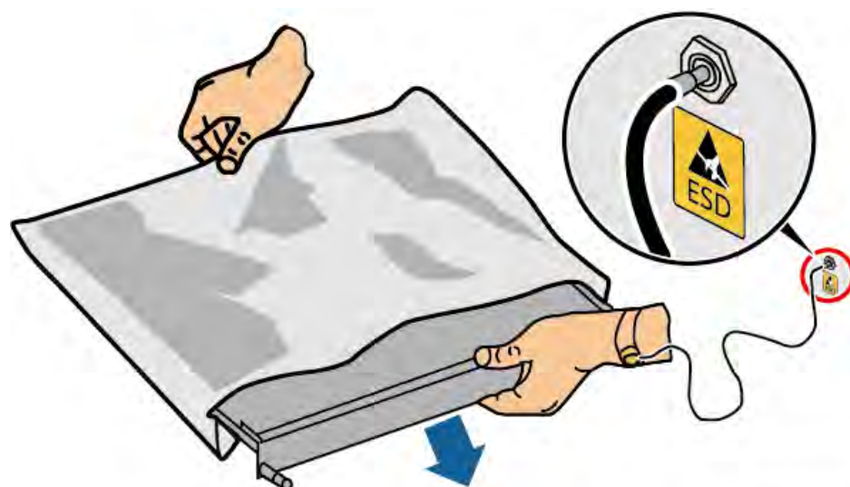
Figure 1-2 Wearing an ESD wrist strap
