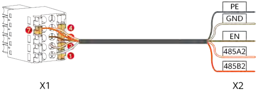
Figure 6-2 Signal cable (purchased from the supplier, type 1) between the battery and the inverter
